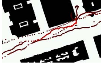
Fig. 6. An uncorrected GPS trace on Marylebone Road
