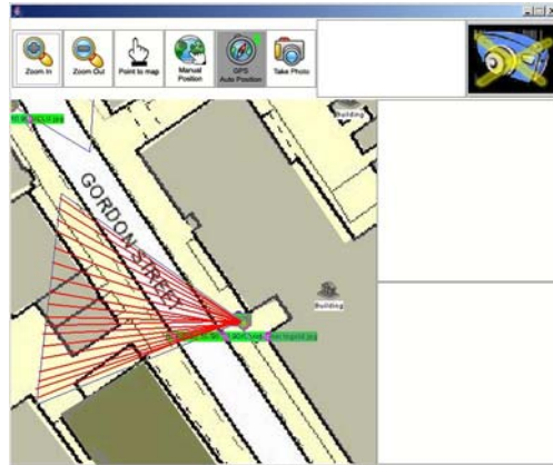
Fig. 2. Example of raycasting approach for associating foci boundaries to photographs. The lines originating from the photograph icon indicate some example rays that are cast from the photographs location. Note that because of the direction the photograph is taken in, the photograph is not associated to the closest building which is ‘behind’ the camera
